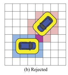
Figure 2. (a) The vehicle's space-time request has no conflicts at time *t*. (b) The black vehicle's request is rejected because at time *t* of its simulated trajectory, the vehicle requires a tile already reserved by another vehicle.
