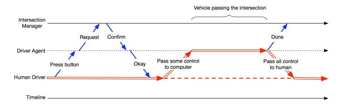
Figure 5. The interaction between human drivers, driver agents, and the IM. The solid lines denote the message passing, while the double stroked lines denote the transfer of control. Note that human drivers retain some control of the vehicle inside the intersection (the dashed line).
