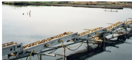
Fig. 2: A number of Miniveyors forms a conveyor line by stacking their endpoints on top of another's.
