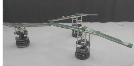
Fig. 1: The prototype of a robot chain network formed by mobile conveyor robots.
